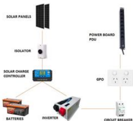
Fig 2 – Off Grid Solar System to power the ICT Equipment.
