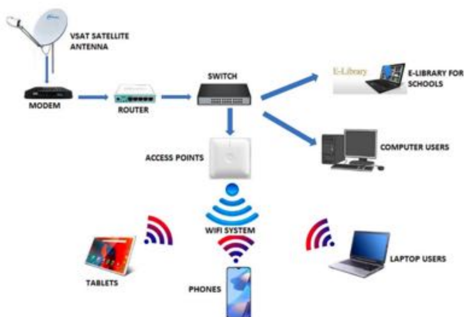
Fig 1 – ICT Services comprising of a VSAT Satellite Internet System, Wi-Fi System.
