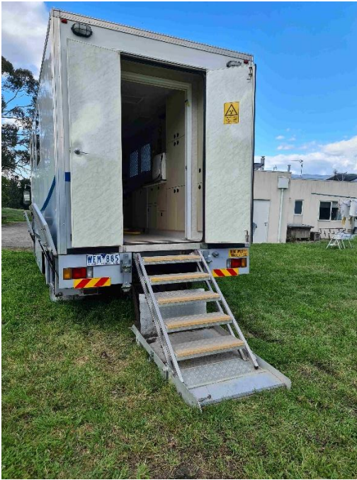
Steps hydraulically raise for safe transport. Separate armrests are provided for access
